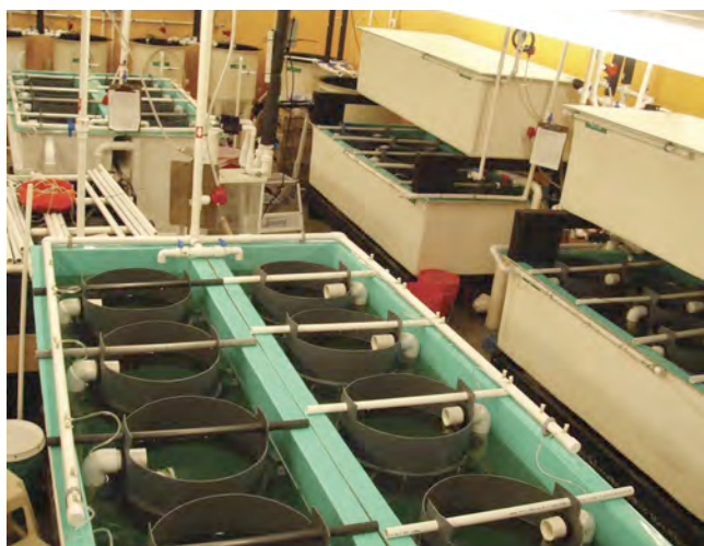
Figure 9a and b. Silos installed in fiberglass tanks are supplied with seawater by airlift pumps and used to hold larval clams during metamorphosis.
