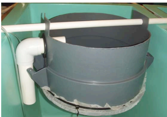
Figure 9a and b. Silos installed in fiberglass tanks are supplied with seawater by airlift pumps and used to hold larval clams during metamorphosis.
