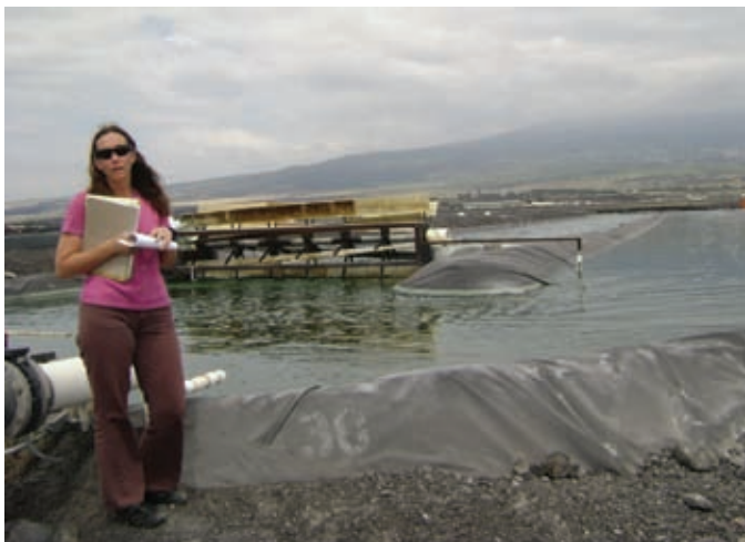
Fig. 7. Cyanotech Director of Business Development Valerie Harmon, adjacent to pond circulated by paddle-wheel and lined with food-grade plastic used to culture spirulina. (Photo by J. Buttner)
