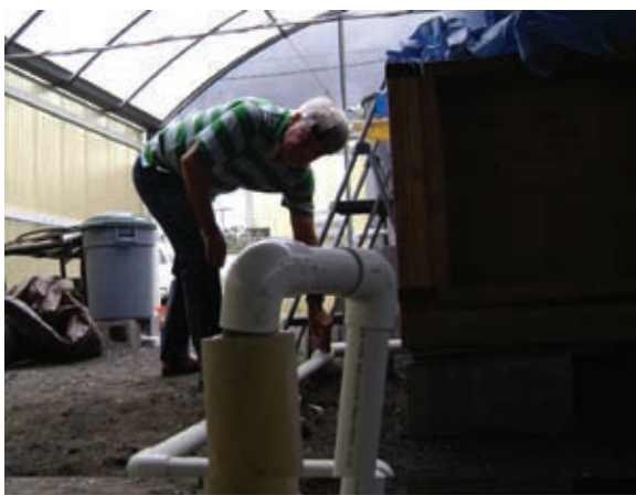
Fig. 7. Jim Szyper, one of four Sea Grant Extension Specialists in Hawaii, flushes accumulated solids from a demonstration recirculating aquaculture system at UH Hilo Panaewa facility. (Photo by J. Buttner)
